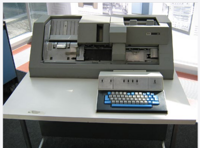
A punch card and a card puncher. A punch card's capacity usually was 80 bytes. 14
